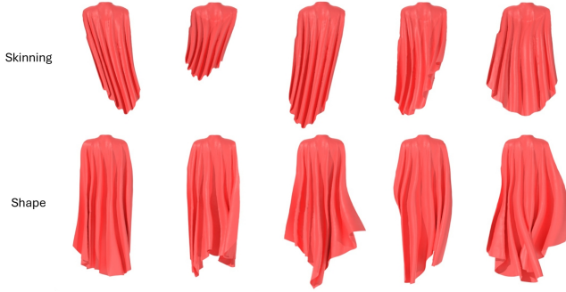
Fig. 8. Top row: first five principle components of the neural skinning PCA model for the cape. Bottom row: first five principle components of the neural shape PCA model for the cape. All of the images depict the augmentation of the rest shape cloth mesh by the PCA displacements, even though the displacements are added to the skinned mesh (not the rest state mesh) during neural shape inference. The PCA model used for skinning tends to capture low-frequency deformations, while the PCA model used for shape inference is better suited for capturing higher-frequency deformations.
